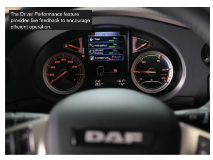
This system evaluates a driver's performance by monitoring a range of behaviours and translates that data into a detailed scorecard. This also provides drivers with tips on how to operate the vehicles to maximise
